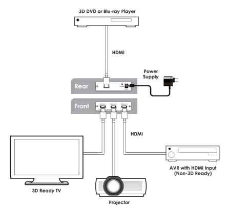
In this example, when the input signal is of 3D format, only HDMI OUT 1 will have picture, while HDMI OUT 2 won't because the projector is non 3D-ready. When the input signal is of 2D format, both HDMI output port 1 and 2 will have picture.
