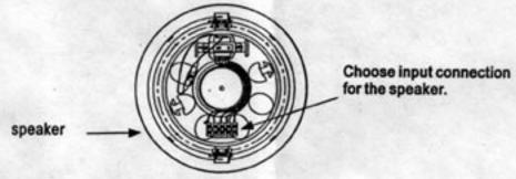
After simultaneously pressing the fixed springs on both sides of the ceiling speaker to the end push it into the round hole of the ceiling and then the speaker is fixed.
