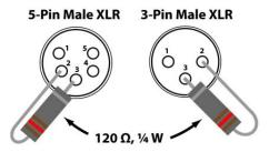
The terminator plug connects to the DMX Out socket of the last DMX product in the daisy chain.
