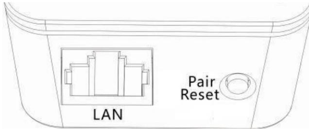
**LAN:** For connecting to the Internet, a PC, or other network device via an Ethernet cable.
