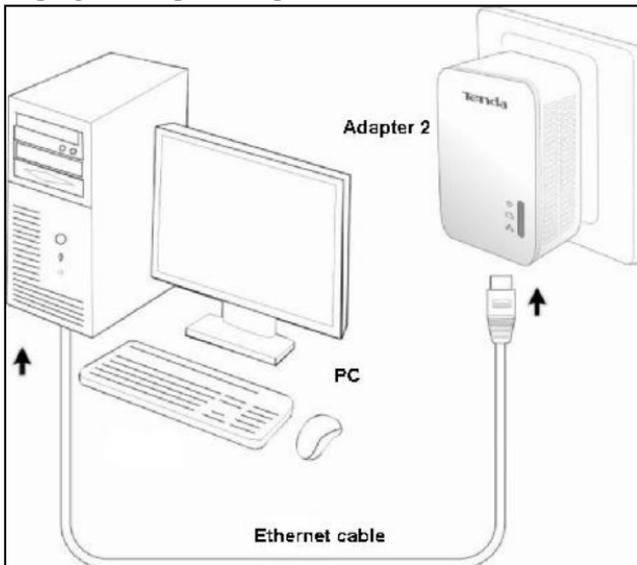
**Step 3:** Once both two adapters are connected to the same power electrical circuit, they are pairing with each other automatically. When both PLC LEDs display solid, the two adapters can access the Internet.
