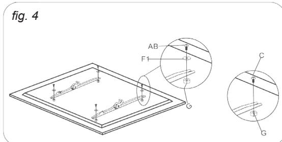
If your screen is curved, use the screws and put a thickness adjuster as shown in fig. 4
