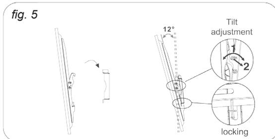
The last step of the mounting consists in fastening the two brackets on the TV back to the bracket you have fixed on the wall and, after adjusting the orientation, lock the screen through the lower screw.
