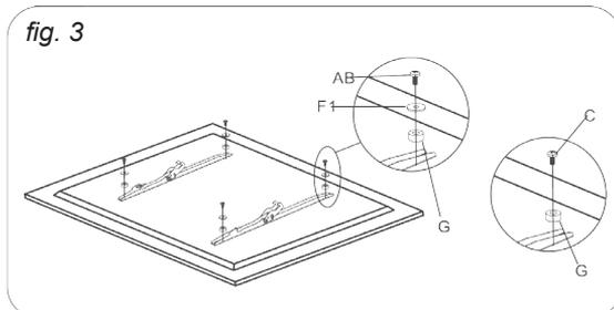
Apply the two vertical brackets to the back of the TV screen making sure to tighten them in the existing TV holes. Refer to Figure . 3
