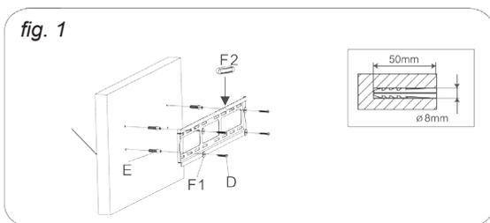
First place the main bracket on the wall, making sure, through the level, that it is perfectly horizontal. Mark the holes with a pencil, make the holes with a drill and fix the bracket on the wall
