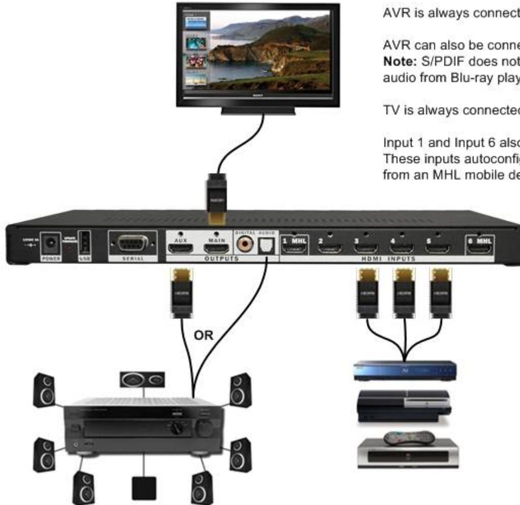
AVR is always connected to the AUX output.
