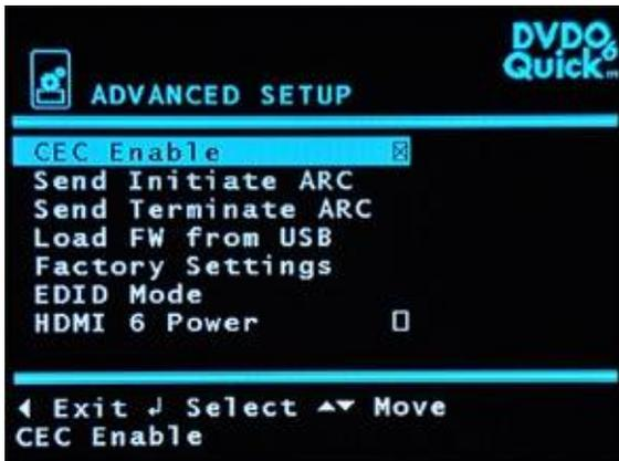
**CEC Enable:** If \*checked, Quick<sup>6R</sup> responds to CEC commands such as power on or off. If unchecked, CEC commands are ignored.
