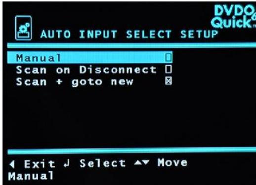
**Manual:** No auto switching; used when Quick<sup>6R</sup> is controlled externally by the serial port or by a universal remote.
