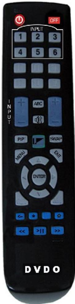
**Power and Standby/Off** buttons are discrete functions that can be taught to any universal remote.
