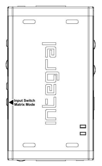
Input Switch / Matrix Mode Button allow you to switch active inputs or enter/exit the Matrix mode.
