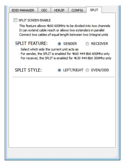
**[SPLIT SCREEN ENABLE]**: This feature allows 4K60 600MHz to be divided into two channels (LEFT/RIGHT or ODD/EVEN) useful for JVC or BARCO and others Dual DVI-D PJ or to extend cable reach or allows two extenders in parallel. Connect two cables of equal length between two Integral units or Integral and Dual-DVI PJ.
