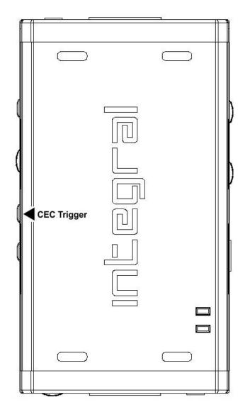
CEC Trigger Button allows you to send two custom CEC commands on the HDMI/CEC network. Integral TOP output port is the CEC master output.
