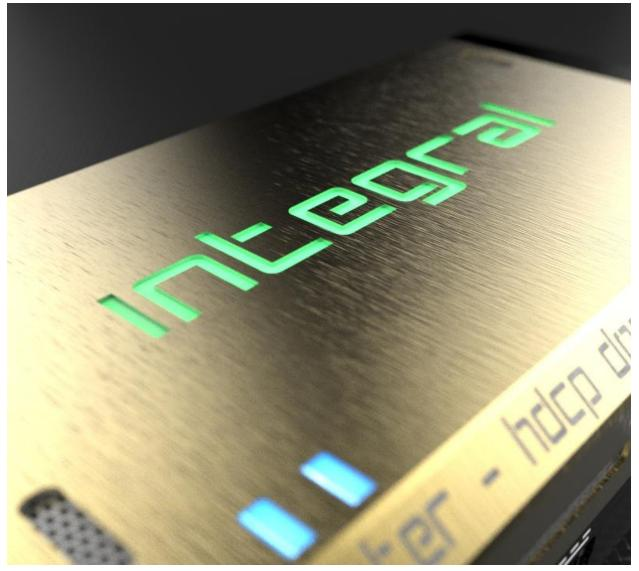
The Integral logo will glow Green when in use. When the Integral first receives an HDMI signal the logo will quickly turn on, then off, and then on permanently to indicate that the HDCP handshake has been completed.
