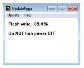
Flashing time is around 50 seconds Do not disconnect your device while the upgrade process is running.
