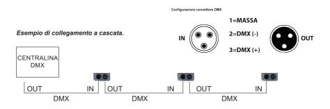
To set the address (from 001 to 512) you want to assign to the unit, press the menu touch (2) until you the letter "d" appears. Then set the address with the keys up and down and confirm with enter. To operate correctly in DMX systems, you have to know the number of channels available in each fixture and the function of these channels. Here is the chart with the functions of the 4 DMX channels of your new fixture.
