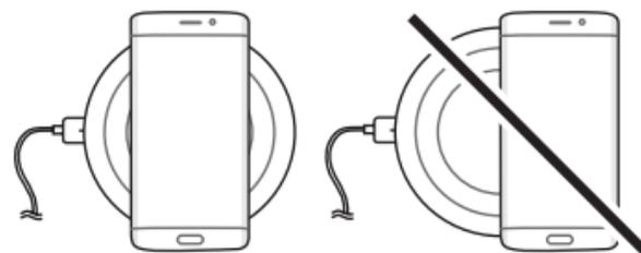
Put correctly your phone in the middle of the charger(a). Wrong position may cause not charging or interruption of it. The leds(c) light on to indicate that the phone is being charged. The leds light off when recharge is completed. In case of false contacts or interruption during charging, please check the correct positioning of the phone.
