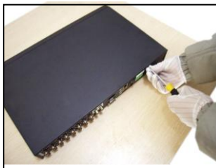
① disassemble the screw
