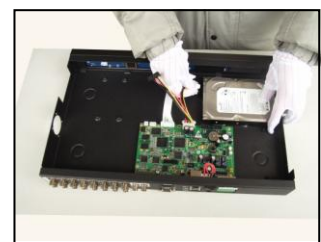
③fix the screw of hard disk
