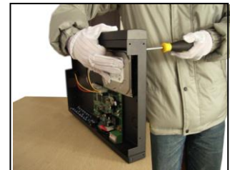
③fix the screw of hard disk
