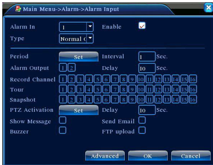
Picture 4.11 Alarm input
