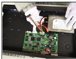
②disassemble the cover
