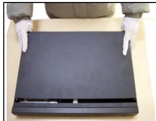
②disassemble the cover
