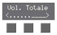
The parenthesis indicate that you are in selection mode; by pressing the side buttons you can scroll through the settings and, by clicking on the central button, you can modify them. When you confirm the settings to be modified, through the pressing of the central button, the parenthesis will disappear and the symbols + and - will appear.
