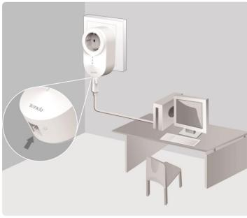
Step 2 Connect the other adapter to a computer, and plug it to a wall receptacle nearby.
