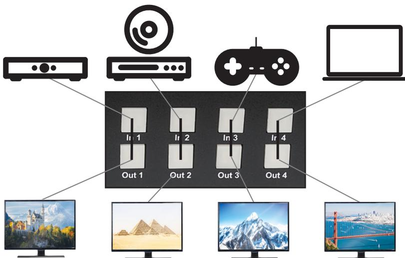
**ENGLISH:** This graphic shows a possible setup of inputs linking to outputs. Each function of this guide references the basic setup shown here.
